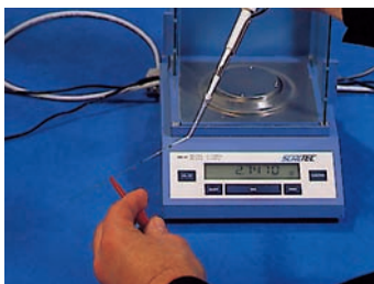
3. Fill the capillary with sample liquid off the pipet tip
