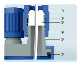
Schematic diagram of GL 45 connection system
