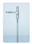
Throughput: 400 l/h at 3.5 bar water pressure und 12 °C water temperature.
