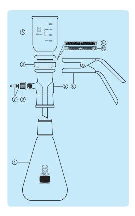
The DURAN® PTFE Adapter combines the ground joint NS 45/40 of the filtering apparatus with the GL 45 screw thread of the DURAN® laboratory bottles. Product benefits: The adapter allows the filtrate to be directly collected in a DURAN® GL 45 laboratory bottle which reduces the risk of contamination. Note: As a vacuum is generated within the bottle during filtration, the use of DURAN® pressure plus+ bottles is highly recommended.
