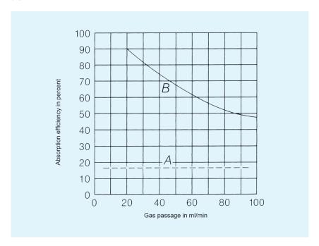
Absorption efficiency of two gas wash bottles: A without gas filter and B with gas filter plate
