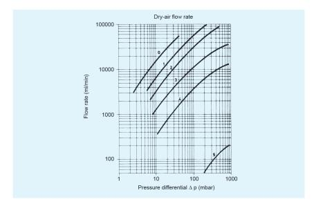
Air flow rate through filter discs of various porosities as a function of pressure differential. For filter discs with Ø 30 mm
