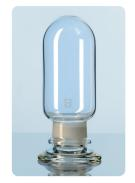
The precise grinding of the knobbed lid and base vessel enables a very tight seal.
