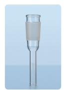
Ground and polished bearing surface, with  ${\sf GL}$  screw thread tube and standard ground cone.
