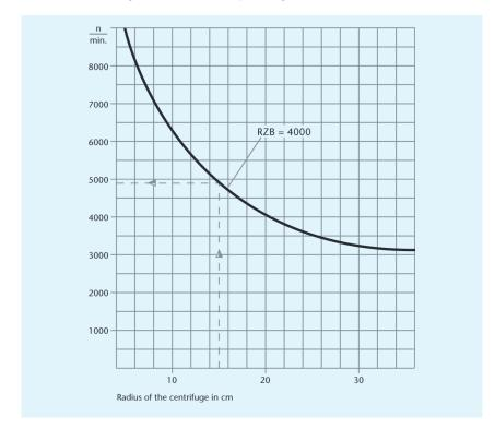
Calculation: RCF =  $1.118 \times 10^{-5} \times r \times n^2$  $n = \sqrt{\frac{4000}{1.118 \times 10^{-5} \times r}}$
